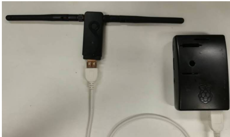
Figure 32: UMOBILE access point HW (Raspberry Pi 3 with Wi-Fi dongle extension)
